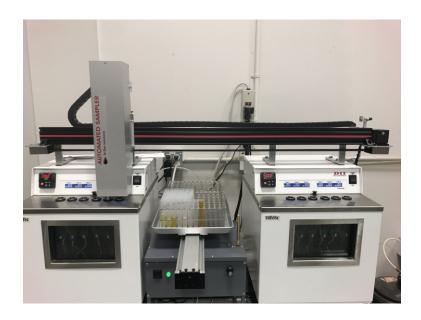
The system is optimized for viscosity measurement of lubricating oils. Ideal for Used Lubricant Analysis laboratories requiring high throughput.
