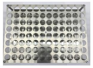
Two of these sample racks (192 samples) may be setup to be run in about 80 minutes.
